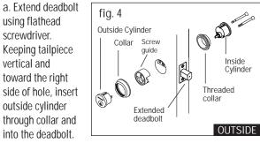
Align slot of inside cylinder with notch in threaded collar. Keeping tailpiece vertical and curved toward the right side of hole, insert inside cylinder with threaded collar into the deadbolt. Attach cylinders using two #10-32 x 2-1/4" flat head machine screws. Tighten screws. Do not insert key during this procedure. (fig.4)
