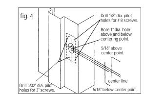
Insert deadbolt into edge of door. While holding faceplate, trace outline of the faceplate onto the door edge. Mark screw hole centers and drill with a 1/8" drill.
