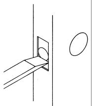
4 Mortise 7/32" deep or until the strike box, reinforcing strike and strike plate fits inside mortise and flushwith the door frame. (fig. 5)
