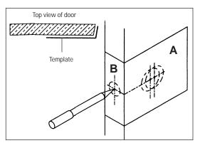
Close door and fig.1 extend deadbolt several times against door frame. Strike centering indicator will leave a center
